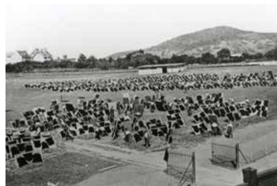
The "panel field" next to the lacquering shop: the panels with patent leather are dried in the sun
